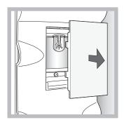
To replace the light bulb in the refrigerator compartment, pull out the plug from the electrical socket. Follow the instructions below. Access the light bulb by removing the cover as indicated in the diagram. Replace it with a similar light bulb within the
